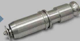
Ring shaped products, based on calamari, onion- or vegetable mix can be easily produced with this special nozzles which form the basis for precise and economic ring extrusion.
