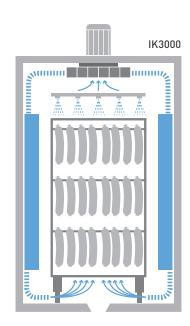
Intensive cooling (natural casing, calibre: 32 mm)
