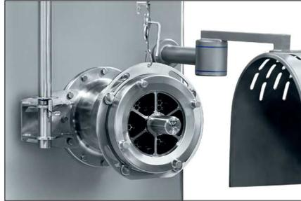
Worm housing nut with smooth running thread and crane
