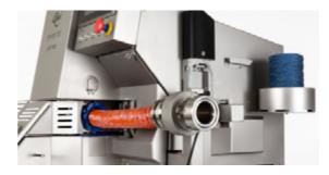
dirt can accumulate, horizontal surfaces with 3° inclines and IP65 rated components. Sealed covers protect valves, drive and controls from water and dirt.
