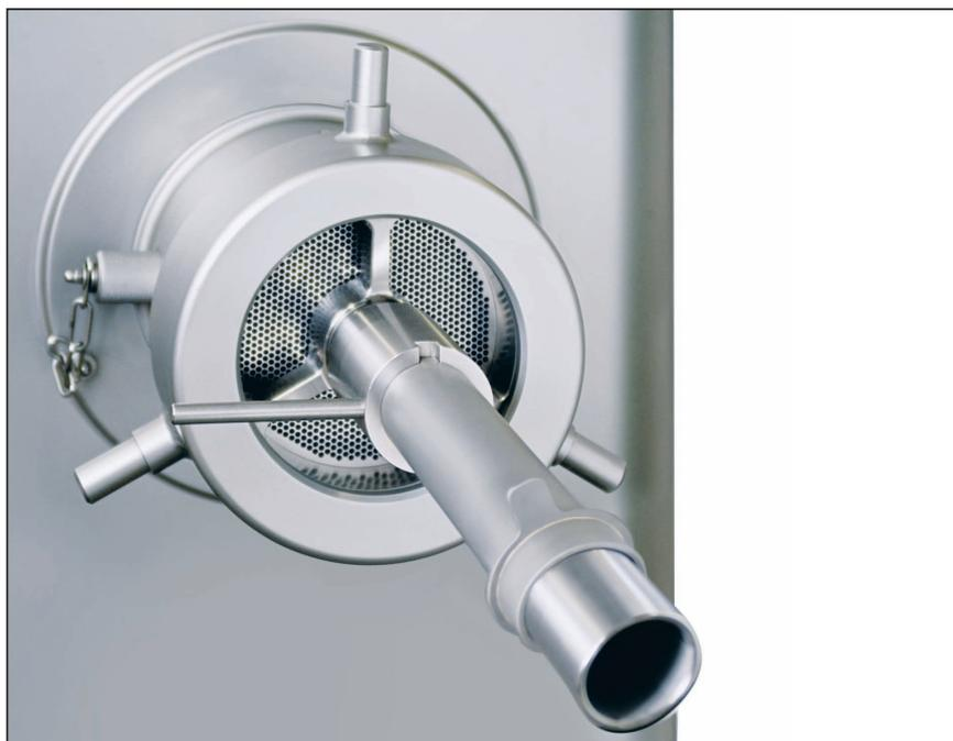
The ULTRA MONO grinders can be equipped with a separator system with lateral outlet and self-regulating spring from cutting set D114 on. The separator systems central and lateral can also be combined. The "Duo Separat" consists of two separating devices which work independent of each other. Thus the separating process can be optimized.
