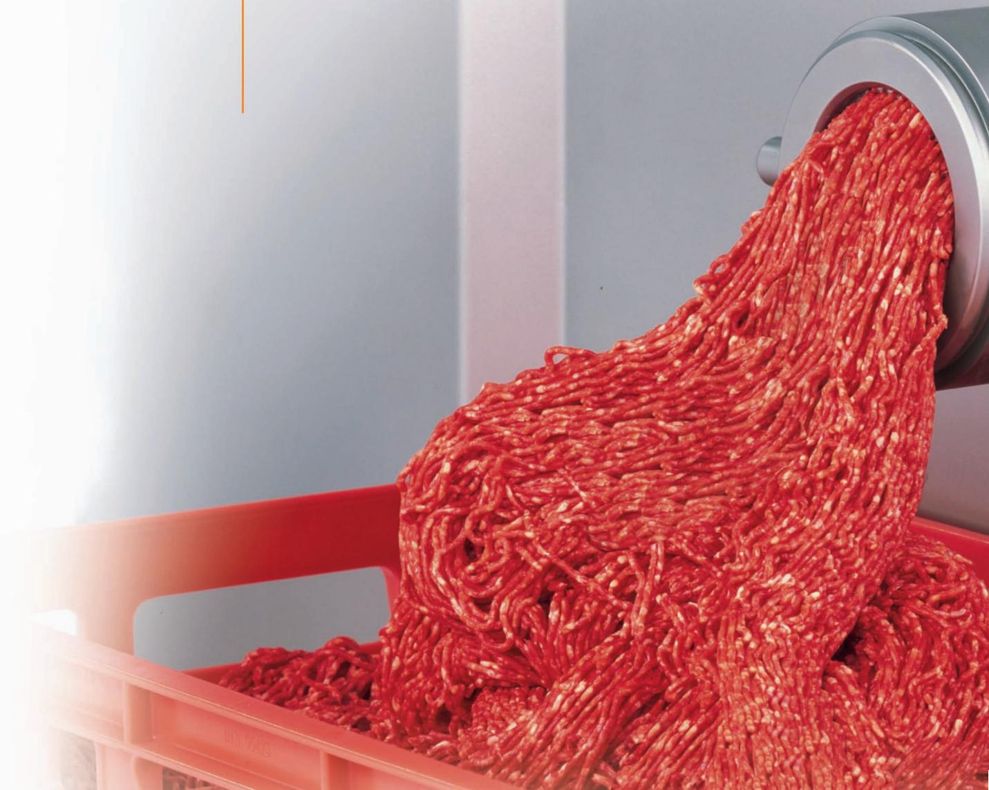
Due to the optimization of the screw geometry and the screw housing and due to the use of new materials, MADO's new MONO grinders achieve top results with peak output in the minced meat production.
