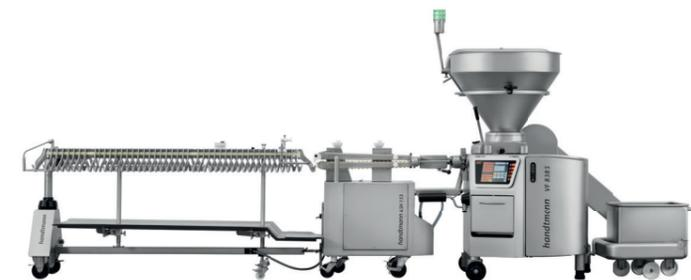
↑ System version for processing natural, collagen and peel-off casing
