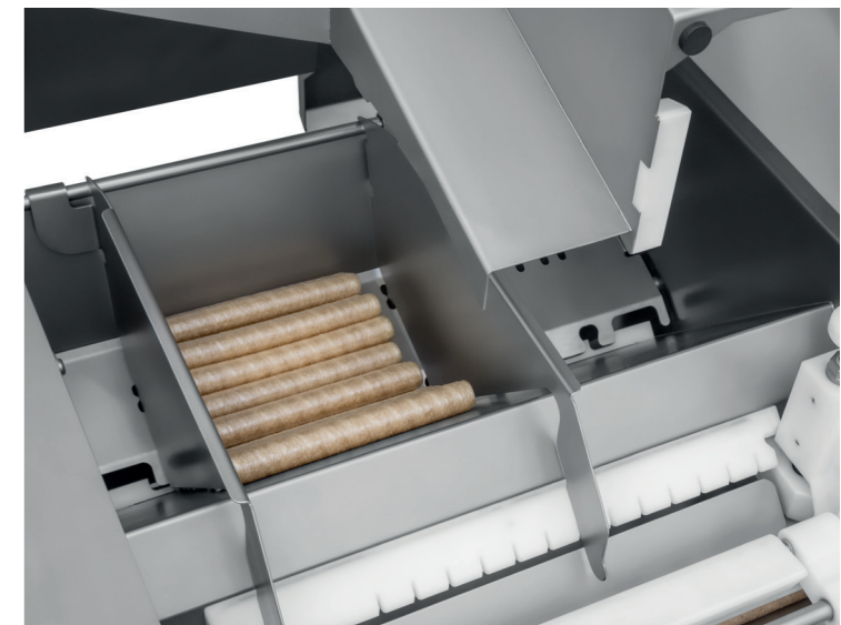
↑ Fully automatic casing change with 3-nozzle revolver and casing magazine ↓
